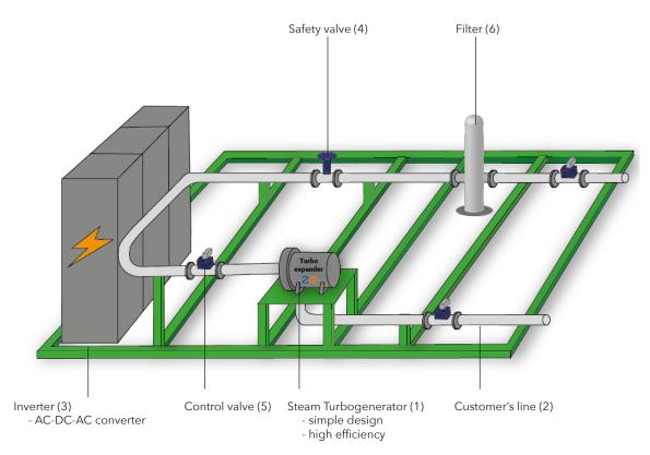
The main part of the steam turbine system is a high-speed Steam Turbogenerator (1), which comprises a back-pressure turbine and a generator placed on the same shaft. The high-pressure steam from the boiler (steam generation device) is directed to the Steam Turbogenerator.
