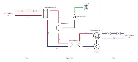
A heat source [1] generates heat that is transferred through a vector fluid circulating in a closed loop to one or more primary heat exchangers, usually a preheater and an evaporator [2], where heat is transferred from the vector fluid to the working fluid.
